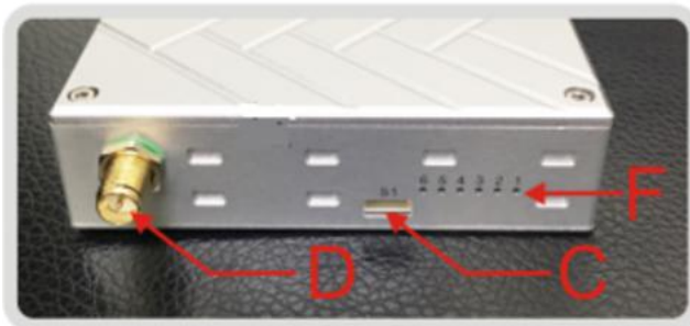
C: 1*TTL 232 Bidirectional Serial Port D: 1*SMA Antenna Port F: Working Station Indicator
