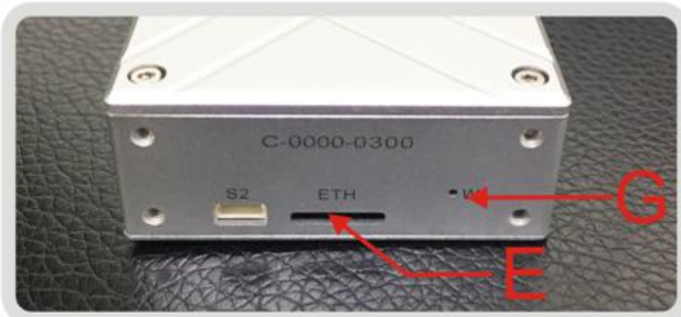
E: 1*100Mbps Ethernet G: WL Signal Indicator
